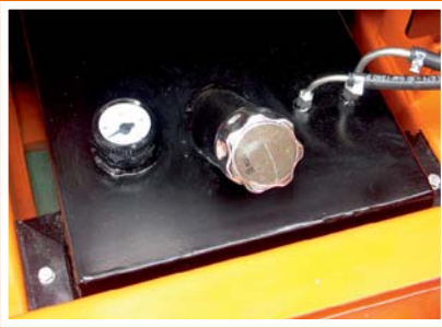
Fuel tank with level gauge
